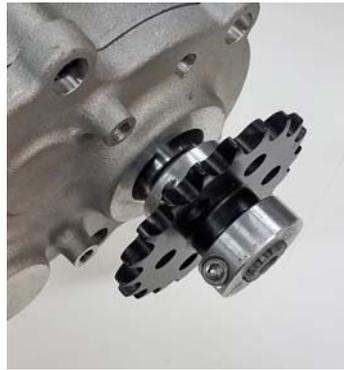
Step 5. Slide on the 3/4" split collar and then slide on the splined sprocket either hub first, or vice versa, and then screw in the retaining bolt and washer. Slide the split collar up against the sprocket for the desired endplay. You can also use two of the split collars to locate the sprocket. You
